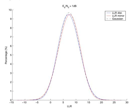
Figure 5: The adjusted LLR distribution is asymmetric  $(E_b/N_0 = 1 dB)$ , other conditions are same as Figure 1(a)). The blue curve is the actual distribution of LLR, and the red curve is the reflection of the blue one about the mean. The black dashed curve is the Gaussian distribution with the same mean and variance.
