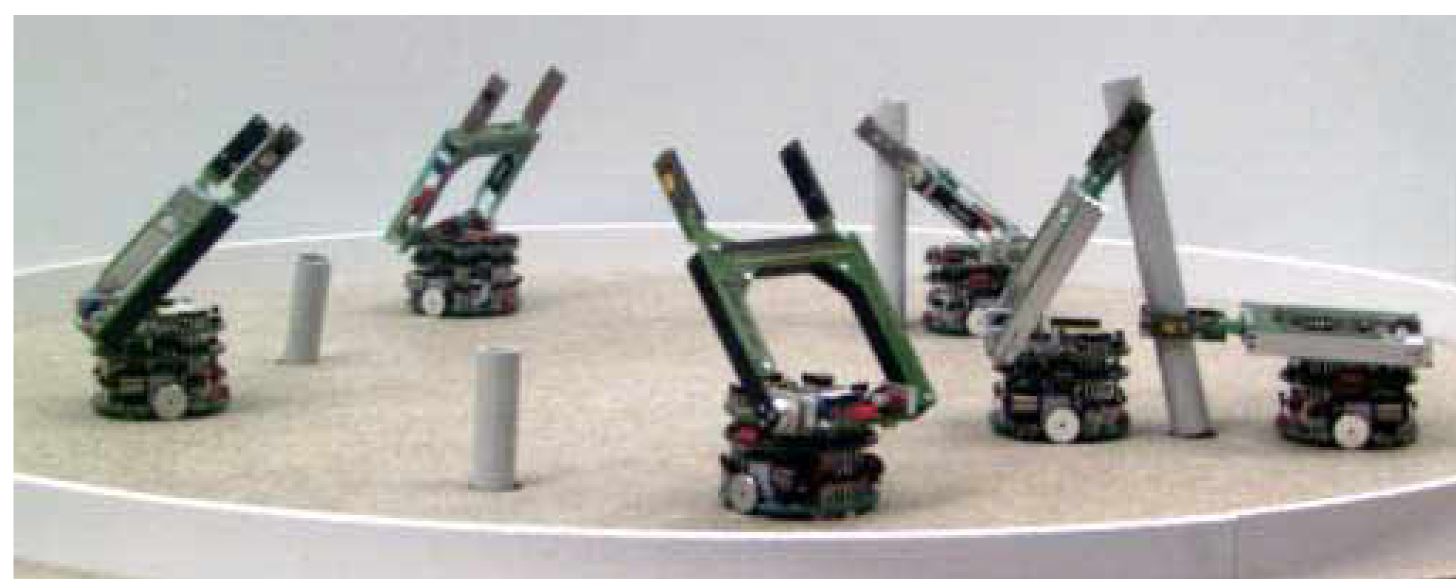
The stick-pulling problem. In the figure, 6 robots with gripper turrets and proximity sensors are trying to pull sticks out of the ground. The stick is long so that one robot can not pull it out by itself. They need collaboration. The gripping time is the time a robot will wait while holding a stick.
