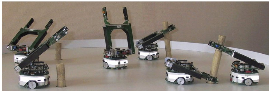
Figure 2.1: Physical set-up for the stick pulling experiment. Collaboration between two robots is necessary to pull a stick out of the ground.
