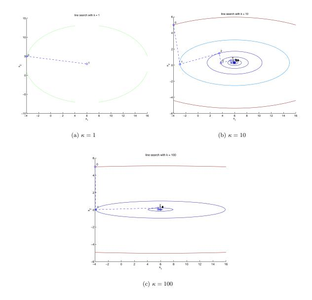
Figure 1: Line search with  $\kappa = 1, 10, 100$ . The small circles with numbers are  $x_k$ 's, and the dashed lines give the descent direction  $p_k$ 's. Those ellipses are contours of the object function.
