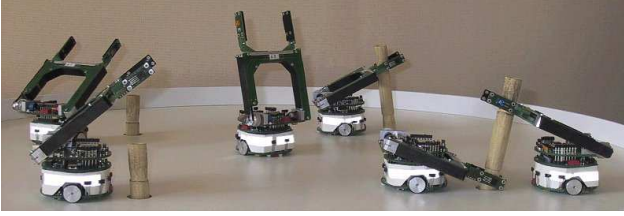
Figure 2: Physical set-up for the original stick-pulling experiment. Collaboration between two robots is necessary to pull a stick out of the ground.
